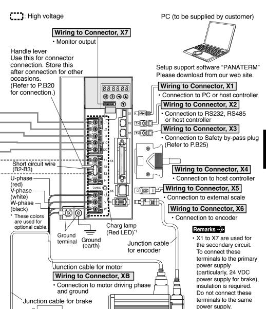
\*1 Do not make displacement, wiring or inspection while the LED is lit - cause of electric shock.
