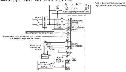
Note For wiring the motor connector, refer to P.B23.
