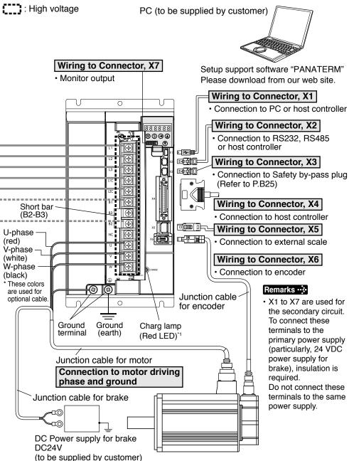
\*1 Do not make displacement, wiring or inspection while the LED is lit - cause of electric shock.
