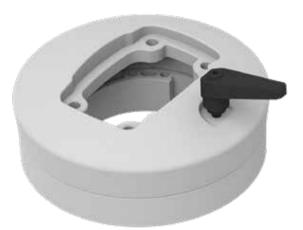
ARM080.320 Rotatable Panel Coupling provides the connection between the operator arm and the operator panel. The diameter is 133mm with a rotation capacity of 315° allowing the operator to rotate the panel to any desired position. It is produced for panel types with high depth ratio.
