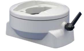
ARM080.830 Rotatable Panel Adaptor Vertical is the connector between the operator panel and the operator arm. The dimension of the adaptor surface is 118x65mm which allows a 315° smooth rotation to the left and right. This product is designed for medium loads and a suitable depth ratio.
