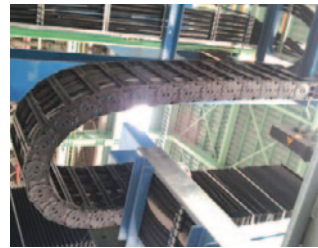
ST095N Application : Production lin for steel products Country : South Korea Remark : Available various stroke and moving direction
