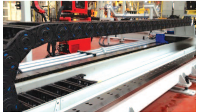
ST120N Application : Robot carriage line Country : China Remark : 3M stroke application
