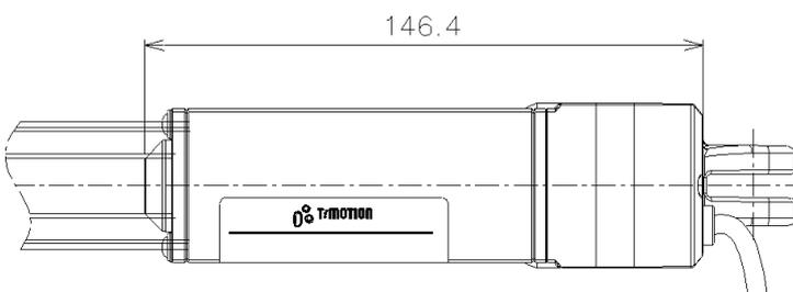
**C. Dimensions - with POT for Load and Speed Code A, B, C, D (mm)**
