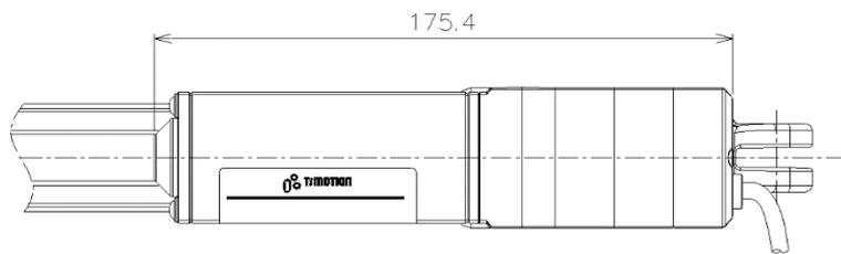
**D. Dimensions - with POT for Load and Speed Code K, J, G (mm)**
