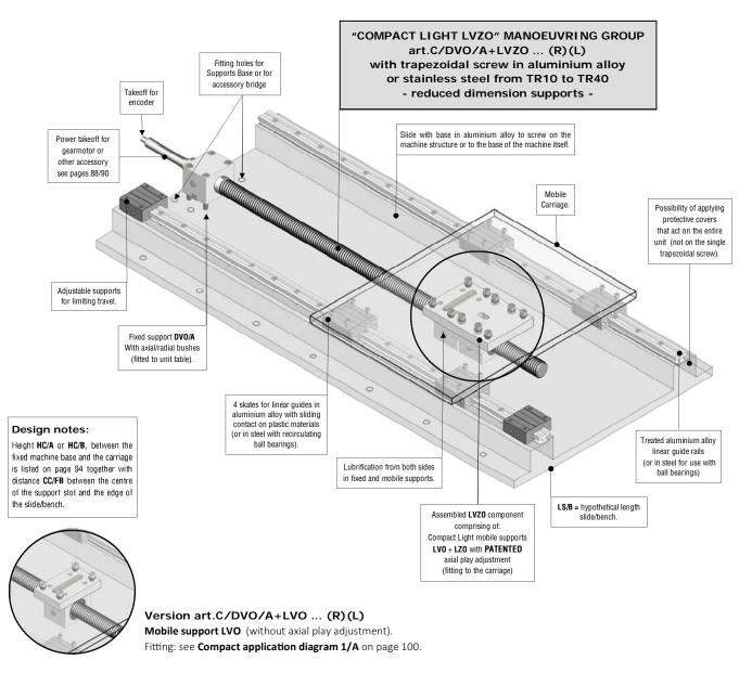
Group with right threaded components available from stock; with left threaded components made to order.
