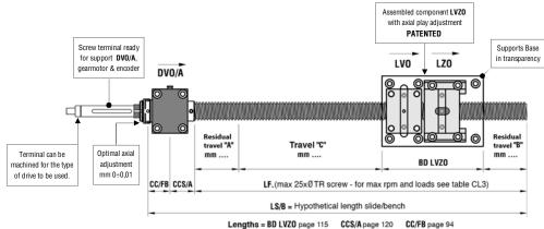
(normally the length BD LVZO is substituted with the length of the entire carriage)
