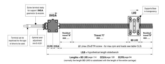
TRAPEZOIDAL SCREW DESIGN of threaded bar ready for the above supports, gearmotor (positioned at the side or above) & encoder. For positioning the gearmotor below (for use only in cases of extreme necessity) please ask for the appropriate screw. Trapezoidal screw terminal: for specific details please see pages 88/90, for general details please see pages 48 - 56.
