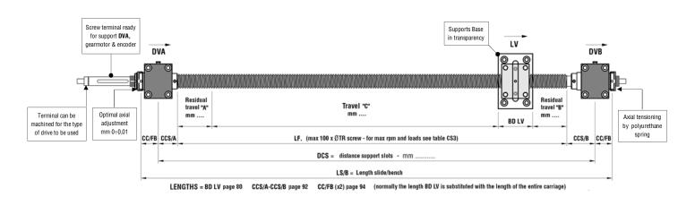
TRAPEZOIDAL SCREW DESIGN of threaded bar ready for the above supports, gearmotor (positioned at the side or above) & encoder.
