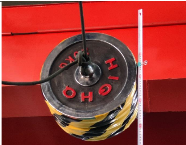
Height of pendulum from the ground during test: 2973 mm 测试中摆锤离地高度：2973 mm
