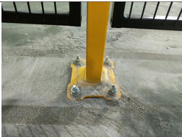
Installation screw of sample after testing 测试后样品的安装螺丝
