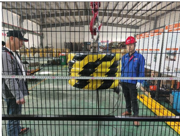
Pendulum hanging in the middle of safety fence: 700 mm 悬在安全围栏中间位置的摆锤：700 mm
