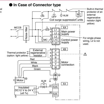
• The pin number of X4 is based on the factory setting parameters.
