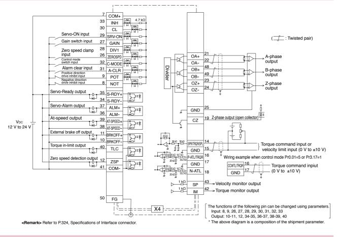
Wiring Example of Full-closed Control Mode
