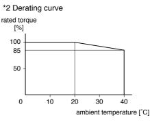
Motor number without \*1, \*2, \*3 Derating curve rated torque
