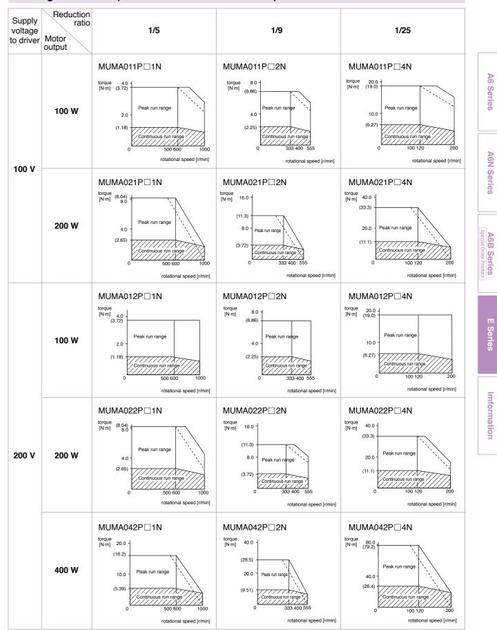
Dotted line represents the torque at 10 % less supply voltage.
