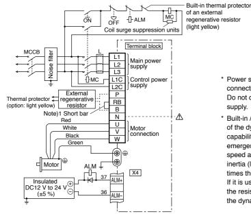
• The pin number of X4 is based on the factory setting parameters.
