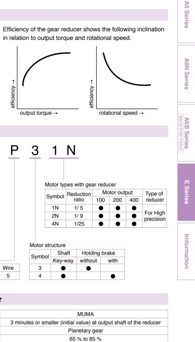
Same direction as the motor output shaft Planetary gear Flange mounting 10 times or smaller than rotor moment of inertia of the motor IP44 (at gear reducer) 0 °C to 40 °C 85 %RH (free from condensation) or less
