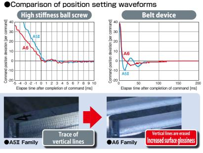
Example of operation with processing machine A mirror finish is obtained even if a process that tends to cause streaking.
