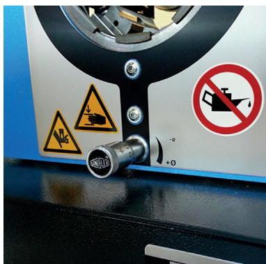
The micrometer allows you to easily set the crimping diameter.
