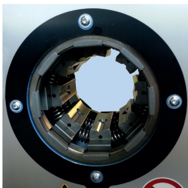
The large opening stroke allows you to crimp all common types of fittings without changing the crimp dies.
